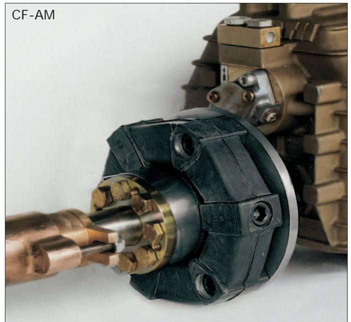
**The CENTAFLEX-M** is available in 2 sizes for 40 and 80 HP approx. depending on propeller shaft speed. Many thousands of these couplings are in service worldwide in motorboats and yachts. Due to the large volume of rubber used, a very smooth transmission of torque and propeller thrust is achieved. The couplings have a fail-safe device which ensures that power can continue to be transmitted even if the rubber fails.
