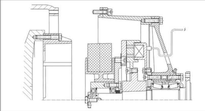
The flywheel flange of the CENTAFLEX-R must be bolted to the flywheel with the correct tightening torque.
