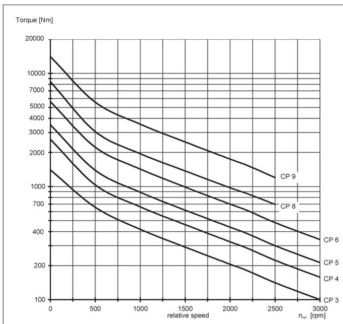
This diagram shows the transmittable torque  $T$  (Nm), depending upon the relative speed (slip)  $n_{rel}$  (rpm) between driving and driven member. The absorbed torque during engaging at a given relative speed must always be lower than this transmittable torque.
